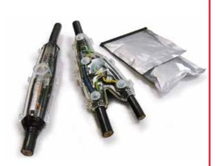
BBC Cellpack cast resin joints offer an overall long-term protection in terms of insulation values and resistance for all kind of cable accessories and cross sections. This is guaranteed by high-grade, unfilled two-component PUR cast resins which are designed for various applications as well as by the shockproof plastic moulds available with or without integrated strain relief. After the hardening process, the cable joints are resistant to mechanical and electrical loads.
